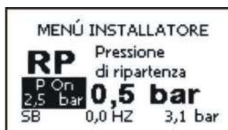
Figure 14: Setting the restart pressure
